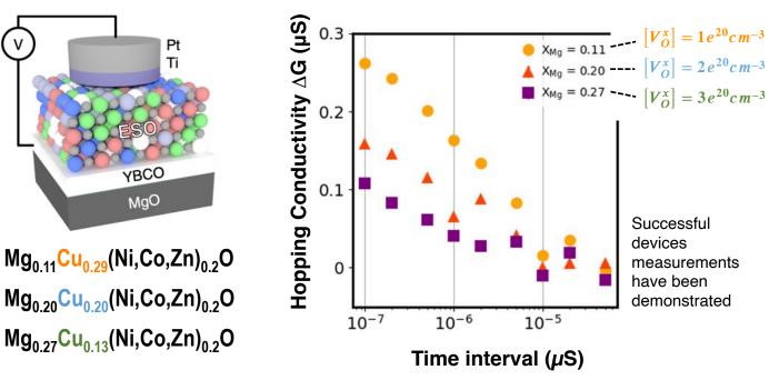
**Left:** Schematic of high-entropy parallel plate memristor device with three different formulations that vary the Mg:Cu ratio, which in turn determines the conduction barriers and relaxation times.
