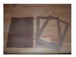
5. Tape the screening onto one of the boards with duct tape; making sure that the screening is pulled tight. This will be your **mold**. The frame without the screening is the **deckle**. Congratulations! You are now ready to begin making your own paper at home!
