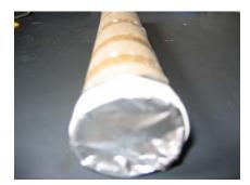
➤ With your pin or needle, poke a small hole in the center of the aluminum foil.
