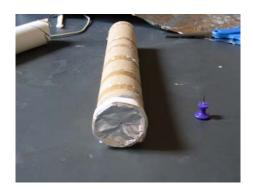
➤ Slide the two tubes together so that the magic tape and the aluminum foil are on the same side. If you slide the little tube inside the bigger one, the clear tape should be next to the foil.
