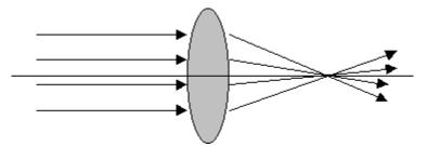
A convex, or converging, lens is thicker in the middle than on the ends. Parallel light rays will meet at a point beyond the lens.
