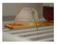
But when you take Nitinol in its higher-temperature form, like in Flexon<sup>TM</sup> eyeglass frames, it is *superelastic*, or very springy. What makes it superelastic is that when you bend it, the pressure that you're putting on the metal causes it to change phases back to its softer form. As soon as you release the pressure, it changes back to its more rigid form.
