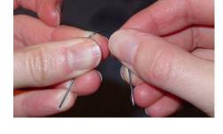
bit, but this makes a huge difference in how the metal feels and behaves. At lower temperatures, Nitinol is soft and easy to bend. At hotter temperatures, it is stiff and springy.
