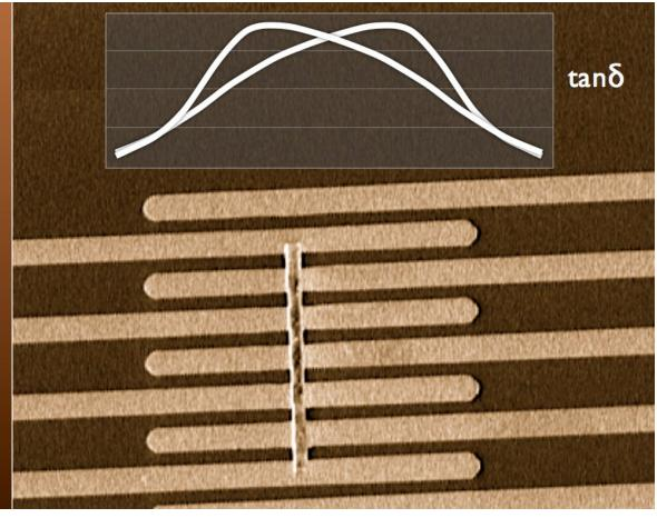
Integrated PZT microtubes provide the first proof of substrate constraints on domain wall mobility in ferroelectric films
