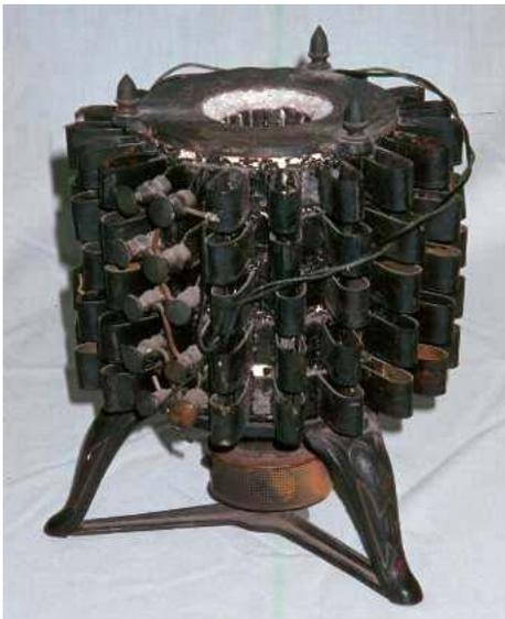
Generators of this type were used ca. 1900 to charge storage batteries. The apparatus is in the collection of Hobart and William Smith Colleges in Geneva, New York.
